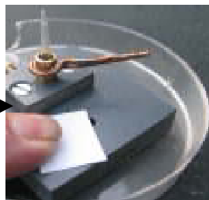
suction control by sliding a piece of paper
